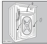
Connect the water inlet hose as described under the paragraph "Water inlet".
